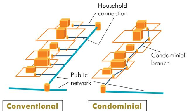
and sewerage. Savings in the volume of soil excavation as a result of shallower trenches were around 45% for water and 75% for sewerage. These physical savings translate into overall financial savings of the order of 24% for the sewerage service and 40% for the water service. This is consistent with recent experience from Brasilia which suggests savings of 20% when condominial designs are used for sewerage systems (Neder, 2001).
